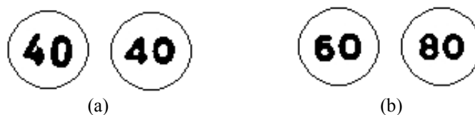
Figure 38. (a) Different representations for the same sign. (b) High similarity between classes.
