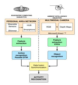
Fig. 1: Block diagram of the overall system.
