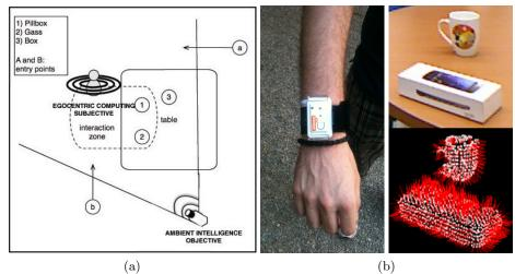
Fig. 2: (a) Setup of the ubiquitous system in a test scenario (b) On the left Shimmer<sup>®</sup> device tied to the arm of the user. On the right, the point clouds with the estimated surface normals of the objects (used in the FPFH object descriptior computation).
