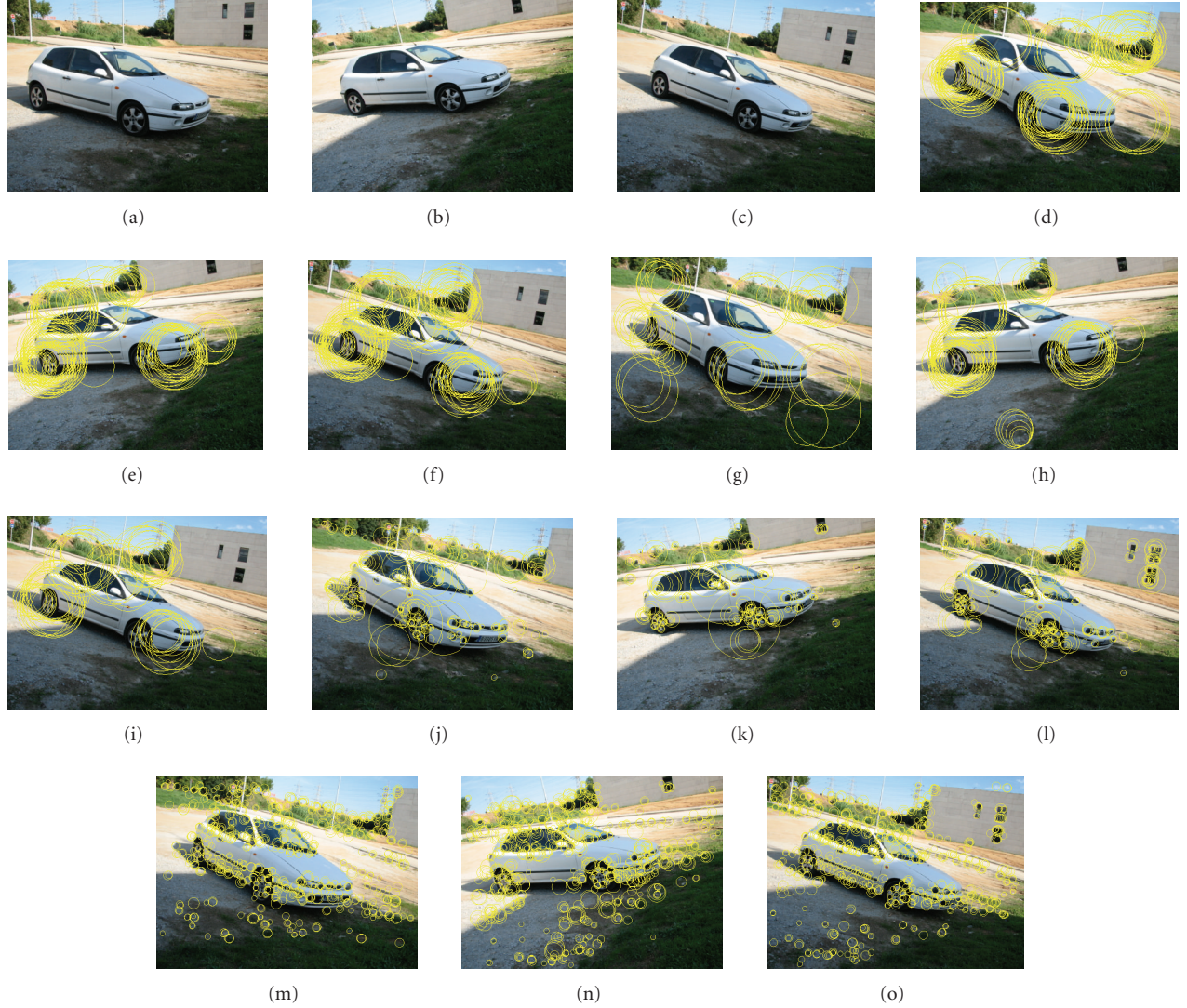
FIGURE 12: (a)–(c) Original images and region detection for (d)–(f) complex salient features, (g)–(i) gray-level entropy, (j)–(l) Harris-Laplacian, and (m)–(o) Hessian-Laplacian for a set of vehicle images from different camera points of view.
