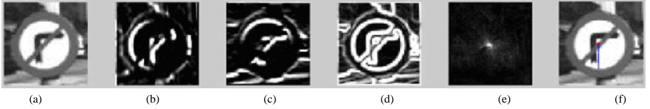
Fig. 3. (a) Input image, (b) X-derived, (c) Y-derived, (d) image gradient g , (e) total orientations accumulator matrix OT, (f) Captured center and radius.
