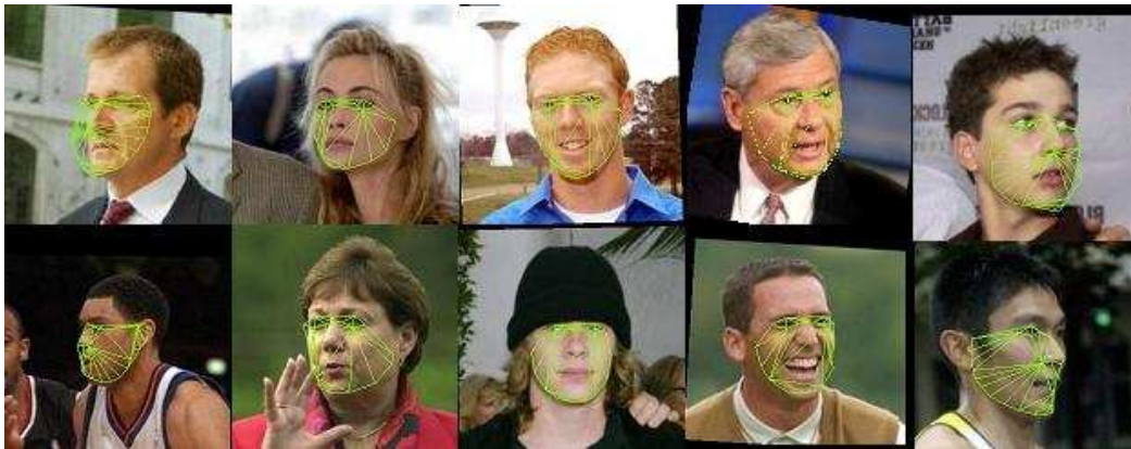
Figure 3: From left to right: left, frontal, and right mesh fitting using AAM.
