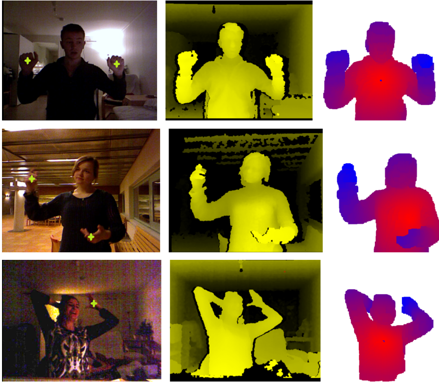
Figure 4. Examples of the data set. From left to right: RGB image and annotated hand locations, aligned depth data, and computed geodesic map applying the proposed procedure.
