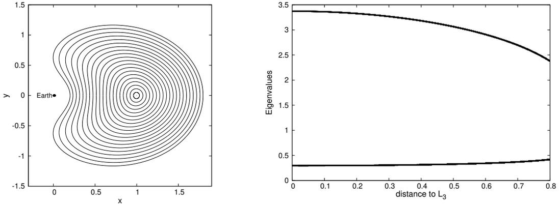
Figure 2: Left: the family of invariant curves around  $L_3$  projected in  $XY$ -plane; the Earth is included as a black circle of corresponding radius. Right: hyperbolic eigenvalues of the invariant curves according to their distance to the periodic orbit replacing  $L_3$ .
