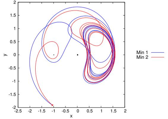
Figure 8: Left, values of the initial conditions in the FCs of Figure 7, that after  $N_T$  BCP periods lay on the position of the asteroid at May 1, 2007, ( $it=14$ ), and the  $\Delta v$  required for each of them. Right, simulation of the capture of the asteroid by the trajectories in the minimum distance areas of the third FC when applying the obtained  $\Delta v$ . The Earth is included as a black circle of corresponding radius, and the initial position of the asteroid as a red star.
