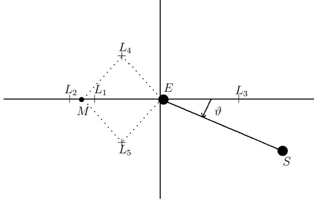
Figure 1: Schematic of the Bicircular Model. Note that distance to Sun is not in scale.
