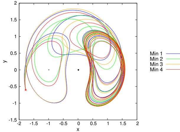
Figure 6: Simulation of the capture of the asteroid at October 7, 2006, through the trajectories in the stable manifold of the fifth FC of Figure 5 when applying the obtained  $\Delta v$ , Table 6. The Earth and the Moon are included as black circles of corresponding radius, and the initial position of the asteroid as a red star.
