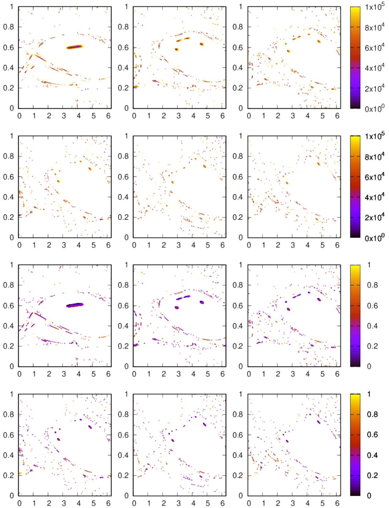
Figure 3: Fundamental cylinders of tori at distances from  $L_3$  between 0.01257 and 0.05784. First two rows, FCs coloured according to the distance to the asteroid at position  $it=2$ , in km, and last rows, same FCs coloured according to the instantaneous  $\Delta v$  in km/s.
