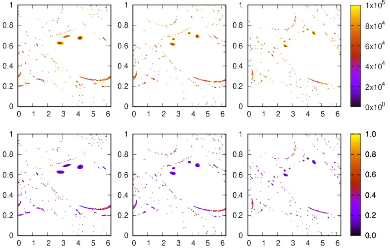
Figure 9: Fundamental cylinders of tori at distances from  $L_3$  between 0.02159 and 0.03947. First row, FCs coloured according to the distance to the asteroid half period after position  $it=3$ , in km. Second row, the same FCs coloured according to the instantaneous  $\Delta v$  in km/s.
