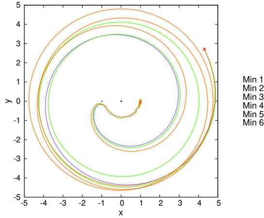
Figure 4: Simulation of the capture of the asteroid at May 12, 2006, through the trajectories in the stable manifold of the fifth FC of Figure 3 when applying the obtained  $\Delta v$ , Table 5. The Earth and the Moon are included as black circles of corresponding radius, and the initial position of the asteroid as a red star.
