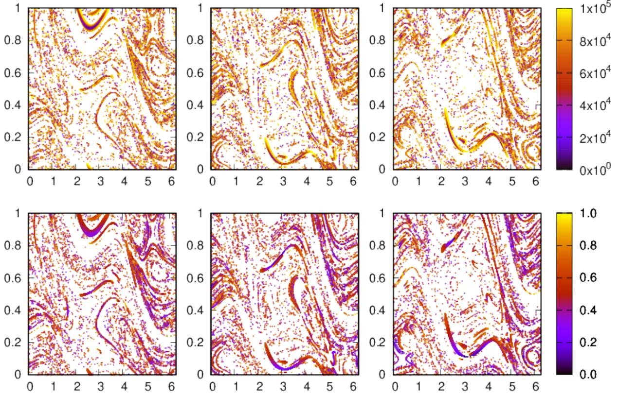
Figure 7: Fundamental cylinders of tori at distances from  $L_3$  between 0.52061 and 0.59139. First row, FCs coloured according to the distance to the asteroid at position  $it=14$ , in km, and last row, same FCs coloured according to the instantaneous  $\Delta v$  in km/s.
