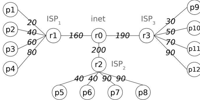
**Figure 4.** Network topology graph. Nodes represent *peers* ( $p$ ) or *routers* ( $r$ )—among different *links* (the arcs). Arc weights correspond to link’s *bandwidths*.
