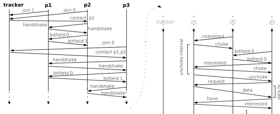
**Figure 2.** Initial stages of BitTorrent simplified protocol. *p* stands for *peer*.
