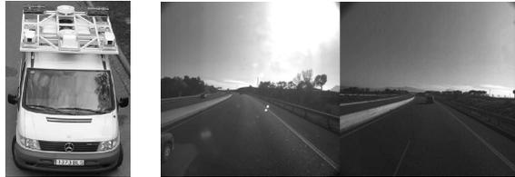
Figure 6. Mobile mapping vehicle and examples of captured images at different conditions.
