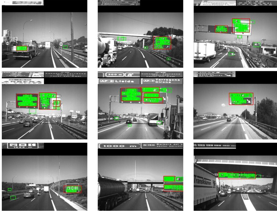
**Figure 8.** Positive text detections from highway images. In this case the text appears in similar conditions. Some text regions corresponds to cars' advertising, and most of the text regions are from information panels. In the top of each image, the content of the detected text regions is shown. The last image shows a false positive detection where the inner structure of the bounding box is close similar to a possible text instance.
