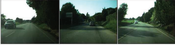
Figure 2: Major challenges for monocular vision-based road detection are the treatment of shadows and the presence of other vehicles.
