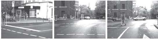
Figure 8: Some detections of the HOG method in the Daimler09 dataset.
