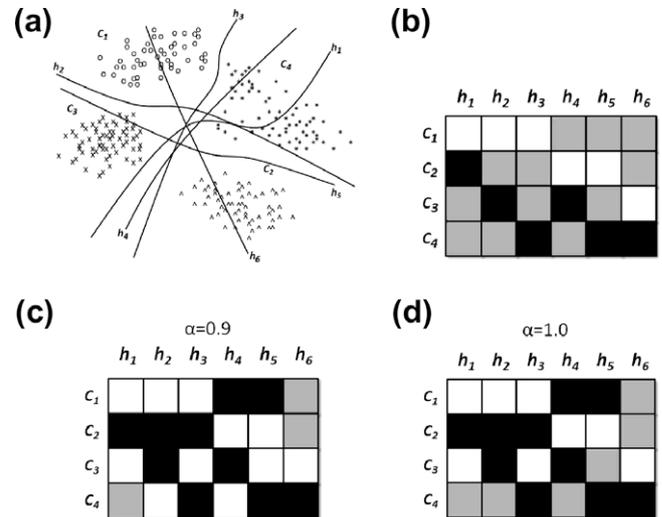
Fig. 2. ECOC codification for a 4-class problem: (a) Non-linear decision boundaries for the 4-class problem, (b) initial one-versus-one ECOC codification, (c) RE-ECOC codification with  $\alpha = 0.9$ , and (d) RE-ECOC codification with  $\alpha = 1.0$ .
