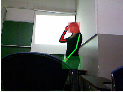
Fig. 4. Upper and bottom agitation. The red dot above the red square represents upper agitation, then the red lines are used to compute the magnitude, while the green dot indicates lower agitation. (The colors are visible in the online version of the article; http://dx.doi.org/10.3233/AIC-140617 .)
