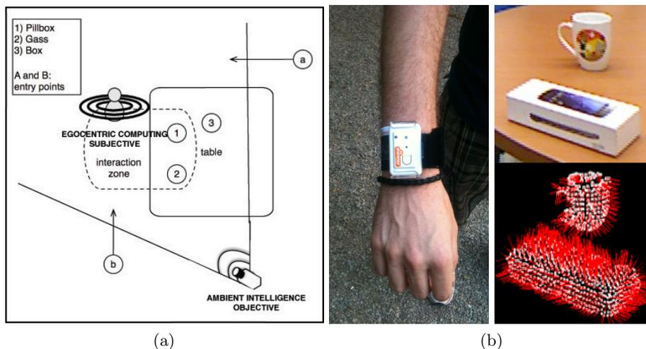
Fig. 2: (a) Setup of the ubiquitous system in a test scenario (b) On the left Shimmer<sup>®</sup> device tied to the arm of the user. On the right, the point clouds with the estimated surface normals of the objects (used in the FPFH object descriptor computation).
