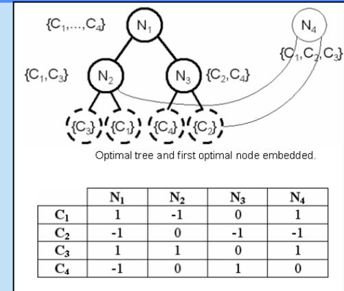
Decoding (weighted attenuated Euclidean distance)
