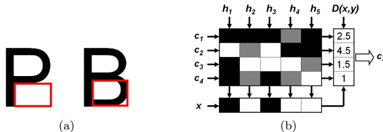
**Fig. 4.** (a) Discriminate features for symbols that shares features. (b) Error Correcting Output Codes coding matrix for a 4 multiclass problem  $\{c_1, \dots, c_4\}$  using 5 binary classifiers  $\{h_1, \dots, h_5\}$ . A test sample  $x$  is tested and classified by class  $c_4$  applying the distance  $D(x, y)$  between the test codeword and each class codeword.
