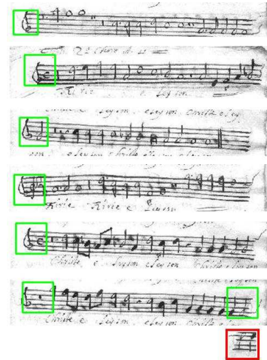
Fig. 4. Clef detection in old stave images. A false positive is shown at the bottom of the figure.
