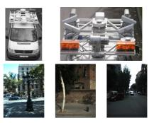
**Fig. 2**. Mobile Mapping vehicle and examples of captured urban scenes.
