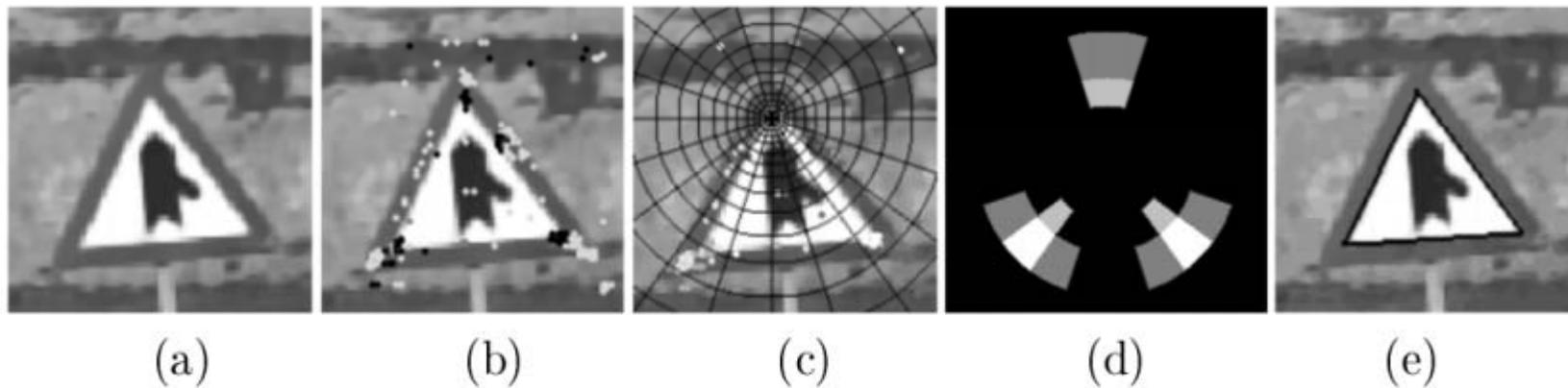
(a) Input image. (b) Detected landmarks. (c) Contextual descriptors. (d) Resulting bins at feature selection of the correlogram of the landmark
