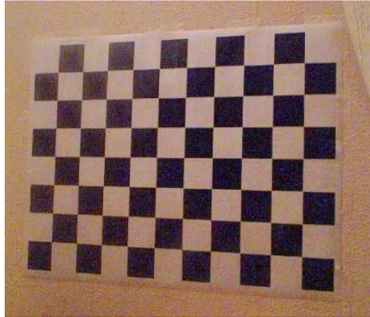
Figure 8.2 2D Calibration template
