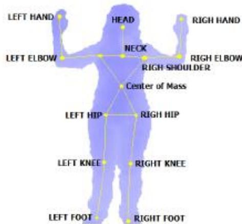
Figure 6.5. Skeletal model formed by 15 joints
