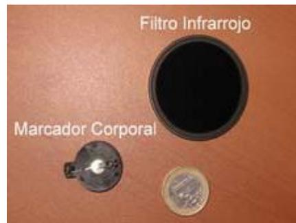
Figure 6.3 Picture with LED markers and cut-off IR filter
