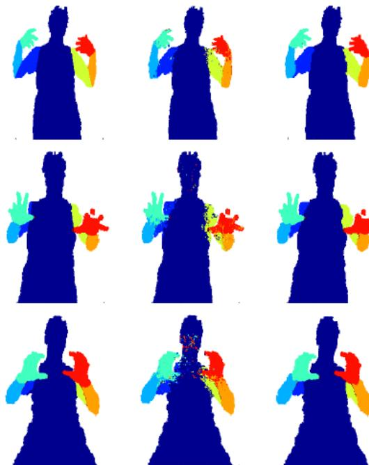
Figure 6.11 From left to right: Depth map Ground Truth and labels, RF inferred results, and GC result over RF output probabilities, respectively
