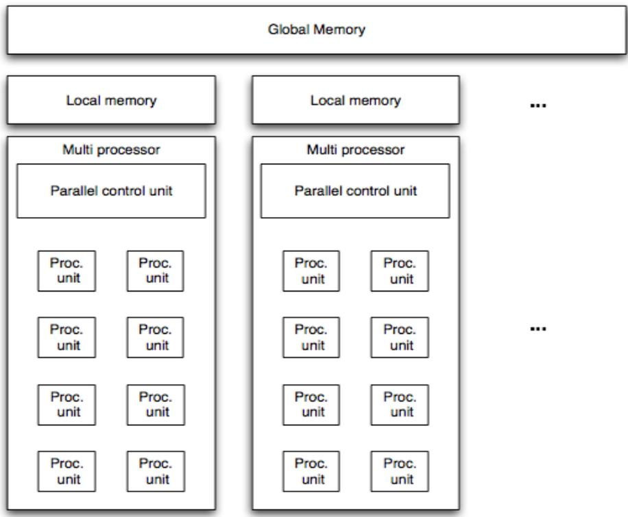
Figure 2.4: block diagram of the general purpose hardware of a GPU.
