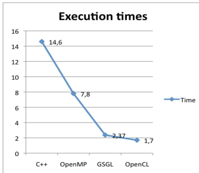
Figure 4.2: execution times for the different implementations of the classification algorithm.
