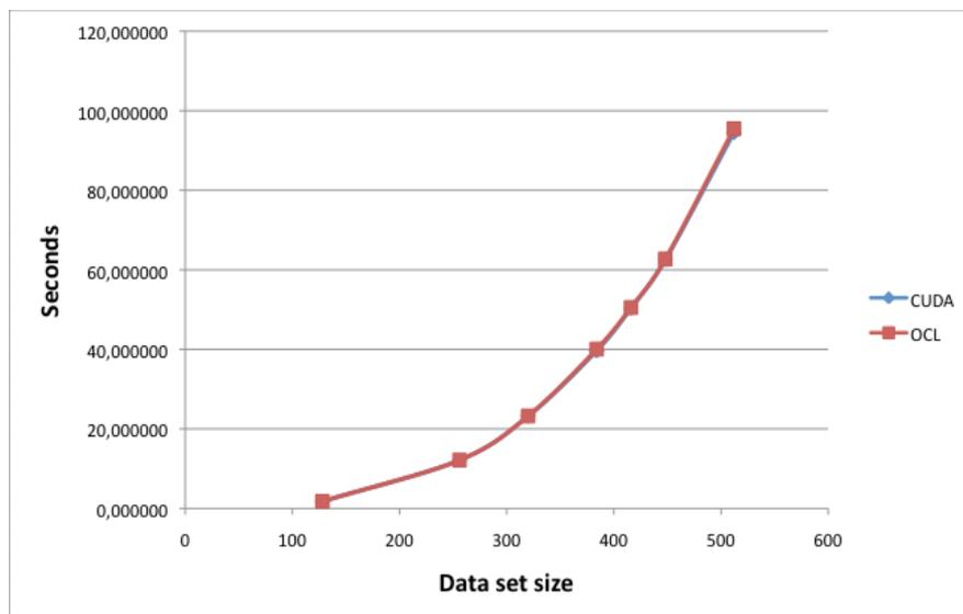
As seen in the graphs, the average difference is almost 0% being CUDA the winner for a very thin margin. So OpenCL for NVIDIA GPU's is still an option.
