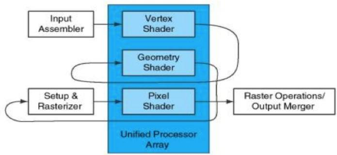
Figure 2.3: representation of the hardware stages computed by the Unified Processor Array [2]
