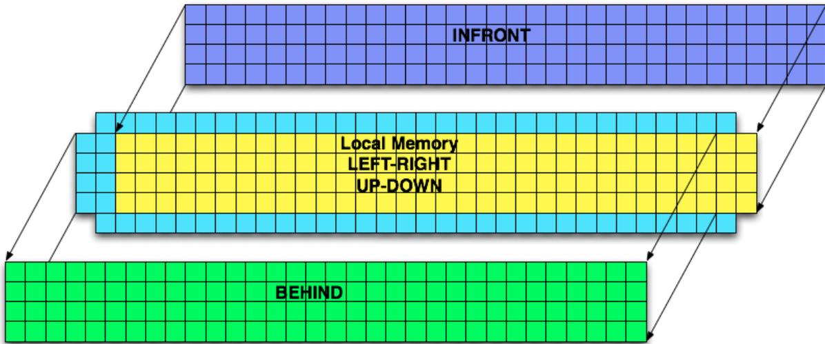
Figure 3.6: representation of the values in registers and local memory for gradient kernel. In yellow values read from infront registers. In blue values read from global memory to local and registers. In green values read from local memory to behind registers.
