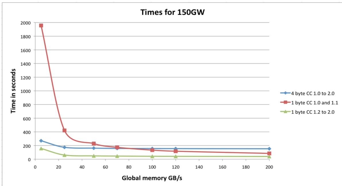
Figure 3.4: Comparing PCIe + global memory theoretical read times with uchar or float types. X axis represents global memory bandwidth in GB/s. Y axis represents time in seconds needed to copy 150GWords from Host to Device and from Global memory to the next memory hierarchy level in gradient kernel.
