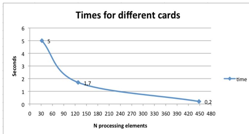
Figure 4.3: execution times for different GPU cards with different number of processing elements. Geforce 9600M GT with 32 PE's, Geforce 8800 GTX with 128 PE's and Geforce GTX 470 with 448 PE's.
