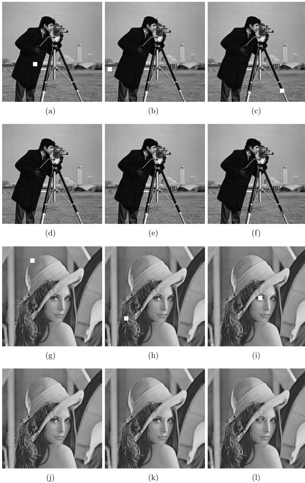
Figure 5.16 Pictures (d), (e), (f), (j), (k) and (l) are the reconstructions of (a), (b), (c), (g), (h) and (i) respectively. The parameters used are 100 iterations, h_0 = 0.5 , \mu_0 = 1 , \alpha = \beta = 1.2 and the squares are of size 10 \times 10 pixels.
